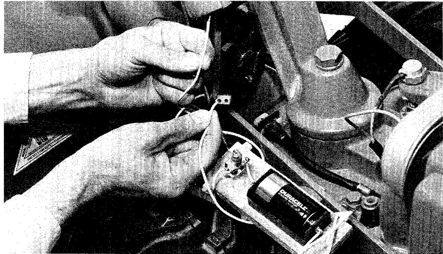
6-79: Test from each terminal hole to bare metal on handlebar.
